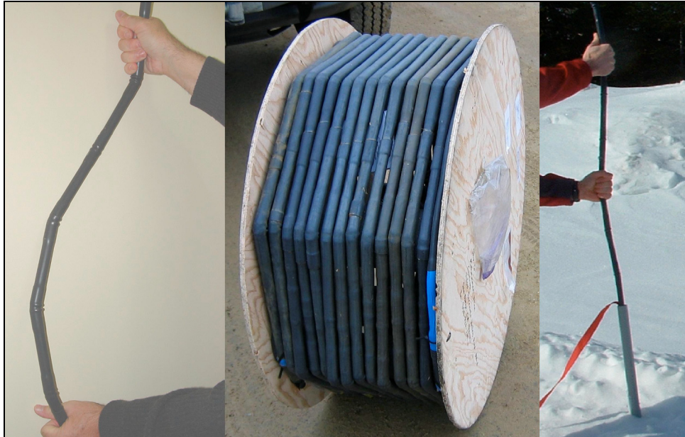
Figure 2: Left: Flexibility of SAA, Centre: SAA on Reel, Right: SAA Inserted into Conduit
